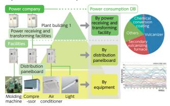
Figure 4: Example of power monitoring level and output
