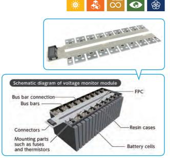
Example of FPC-based voltage monitoring circuit for lithium-ion battery
