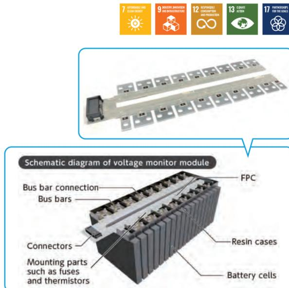
Example of FPC-based voltage monitoring circuit for lithium-ion battery
