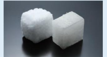
The NOXTITE acrylic elastomer has a number of well-balanced functions, including oil resistance, heat resistance, high strength, and resistance to permanent compression set. In addition to use as a material for oil seals and O-rings, it is used in devices that require heat resistance and oil resistance such as the surrounding surface of car engines.
