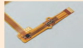
FPCs are very thin films and therefore require a special mounting process. NIPPON MEKTRON not only manufactures FPCs alone, but also responds to requests for FPC module units by mounting semiconductors, microchip components, and connectors.
