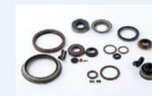
Oil seals are functional parts used to seal oil. Composed of synthetic rubber, metal rings, and springs, they prevent oil from leaking from gaps in machine shafts. They also prevent the entry of dust from the outside.
