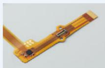
FPCs are very thin films and therefore require a special mounting process. Nippon Mektron not only manufactures FPCs, but also fulfills requests for FPC module units by mounting semiconductors, microchip components, and connectors on them.
