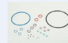
O-rings are O-shaped rubber ring gaskets. They are moderately compressed by fitting into grooves of machinery, and prevent leakage of various fluids, including oil, water, air, and other gases.
