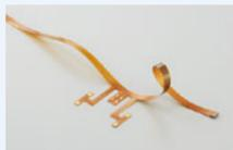
FPCs with circuits on one side are structured to best exhibit their thin and flexible characteristics. They are durable against repetitive bending and can be mounted on moving parts while taking up little space. They are also suitable for multi-dimensional wiring in narrow gaps.
