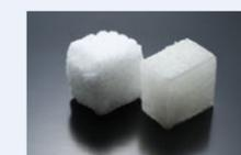
The NOXTITE acrylic elastomer has a number of well-balanced functions, including oil resistance, heat resistance, high strength, and resistance to permanent compression set. In addition to use as a material for oil seals and O-rings, it is used in devices that require heat resistance and oil resistance, such as those adjacent to automobile engines.
